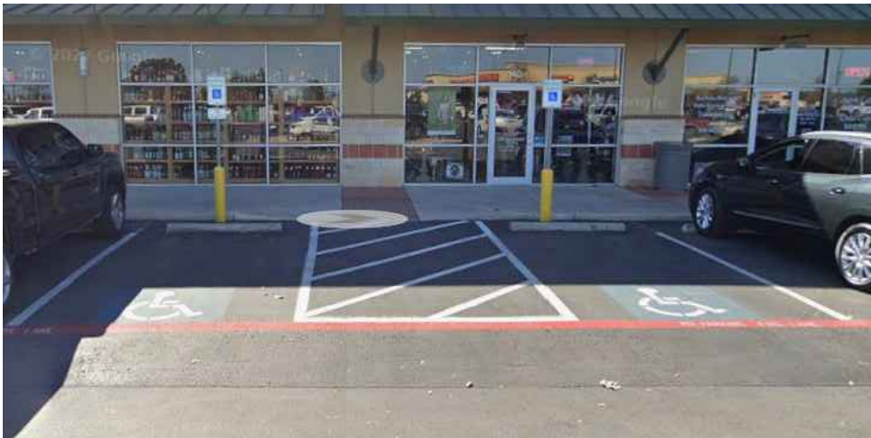
EXAMPLE SITE - TAPERED PARKING SPACES
